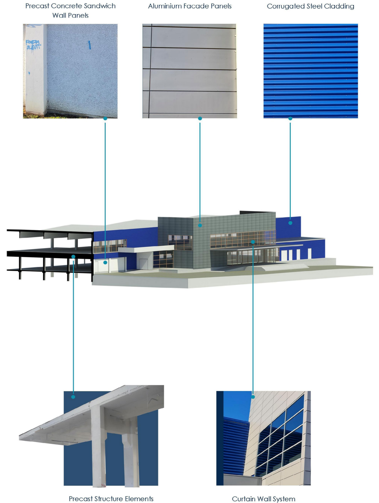
Figure 28. Main types of materials on the existing building.
