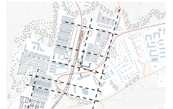
Fig. 67. Potential for improved connections. Global integration is improved by enhancing connections to other areas through Hjällbo and improving internal connectivity (see Hillier and Hansson, 1984).
