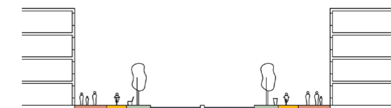
Fig. 109. Central lanes are for higher speeds (3,25 wide and 40 km/h). Cyclists and pedestrians are provided separate lanes (2,5 and 3m) with flexible spaces, including greenery (Stähle et al., 2020). This is proposed for Hjällbovägen as a boulevard with high, motorised traffic.
