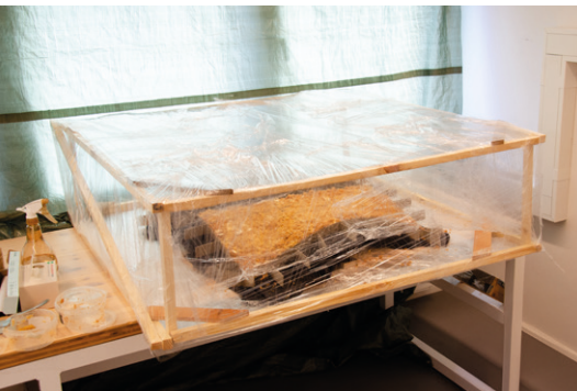
Filled prototype growing in a growing chamber made of wood and plastic 20240428
