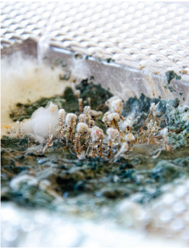
Fig. 10. Contamination and mould is one of the challenges when working with mycelium
