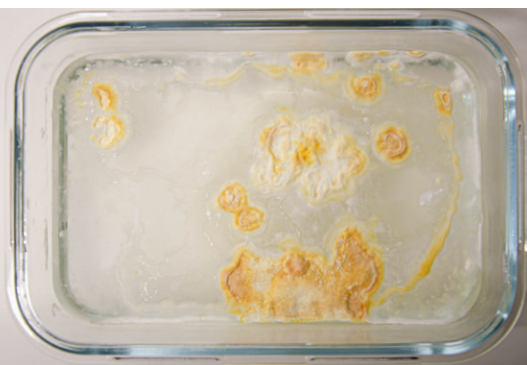
Fig. 12. Mycelium leather growing in liquid livestock (Lab 5.)
