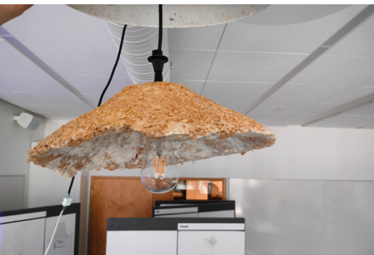
Installed lighting. The mycelium lamp can support itself. 20240513
