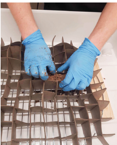
Soaked cardboard mould is filled with substrate, one cell at a time.
