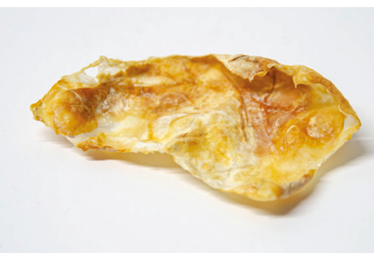
Small sample of heat-pressed mycelium leather 20240509.
