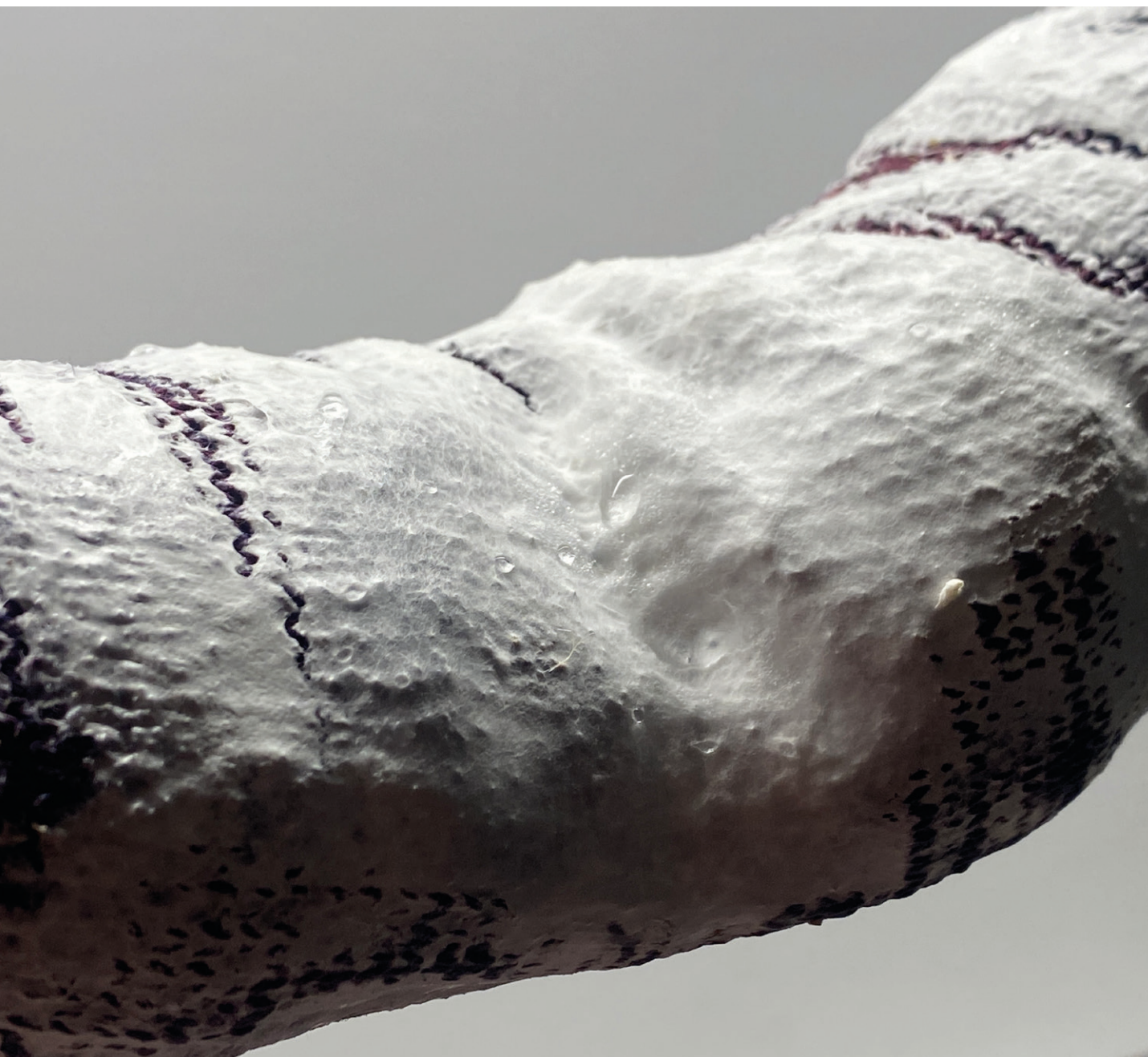
Fig. 19. Mycelium grown in a knitted tube is hang-drying (Lab 9.)
