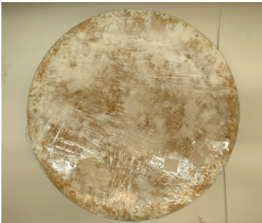
Sample covered with mycelium growth. Some areas has limited growth 20240424
