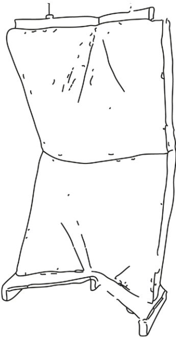
Fig. 16. L'Orso Fungino wall prototype used post-tensioning as a way of stabilising
