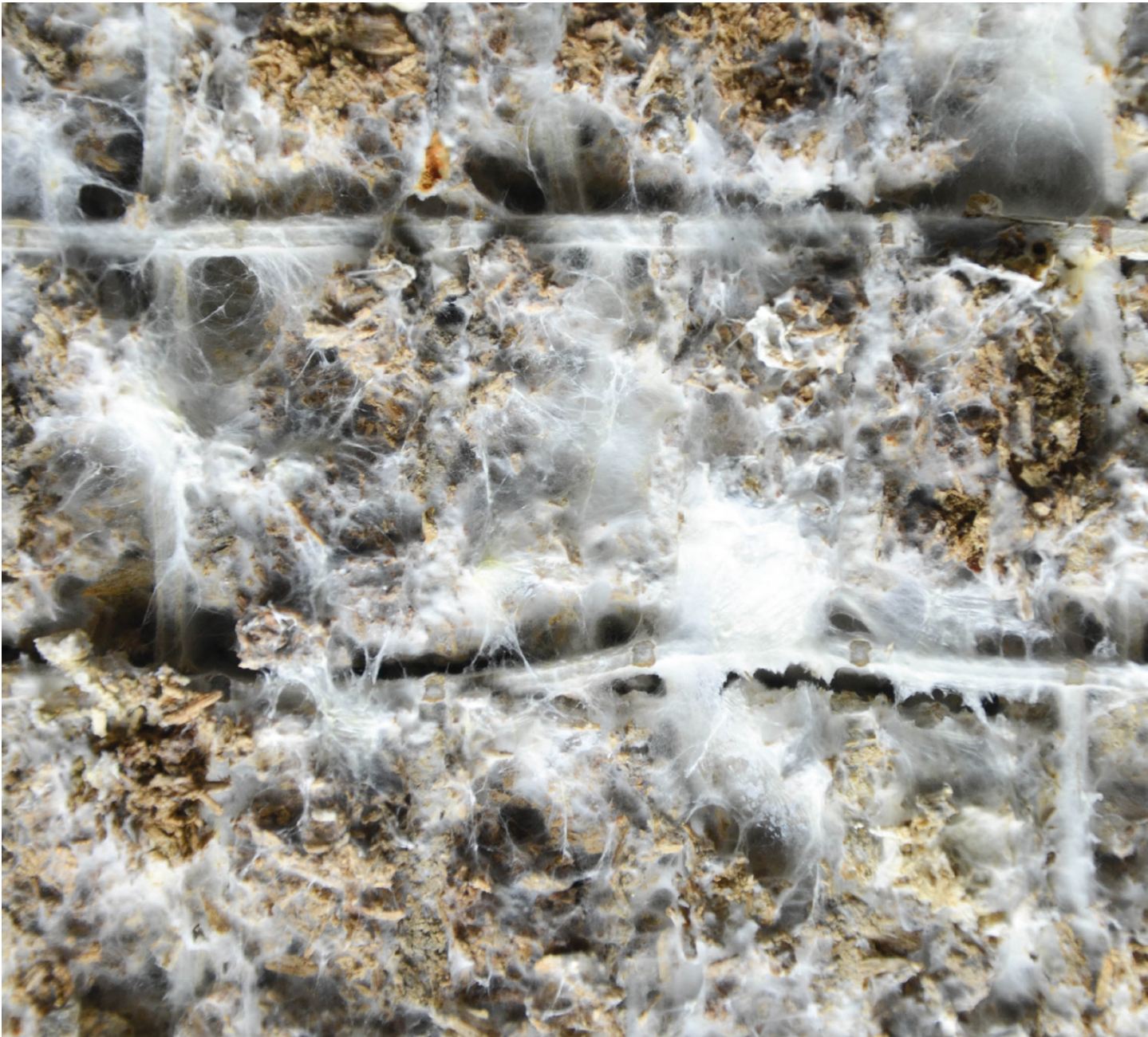
Fig. 24. Mycelium growth on cardboard waffle (Lab 4.)
