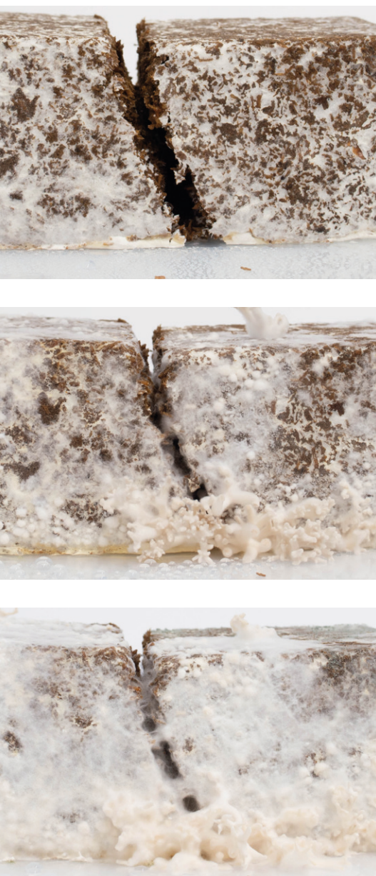
Fig. 08. Mycelium can repair itself (Lab 7.)
