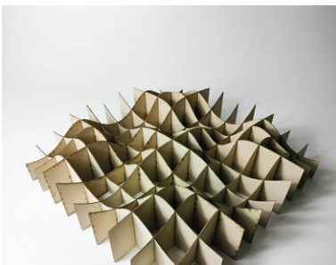
The cardboard waffle mould based on a sinus curved parametric pattern.
