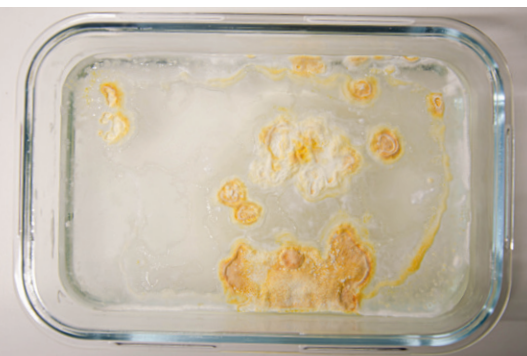
PMM in liquid substrate. Taken out to be heatpressed 20240509
