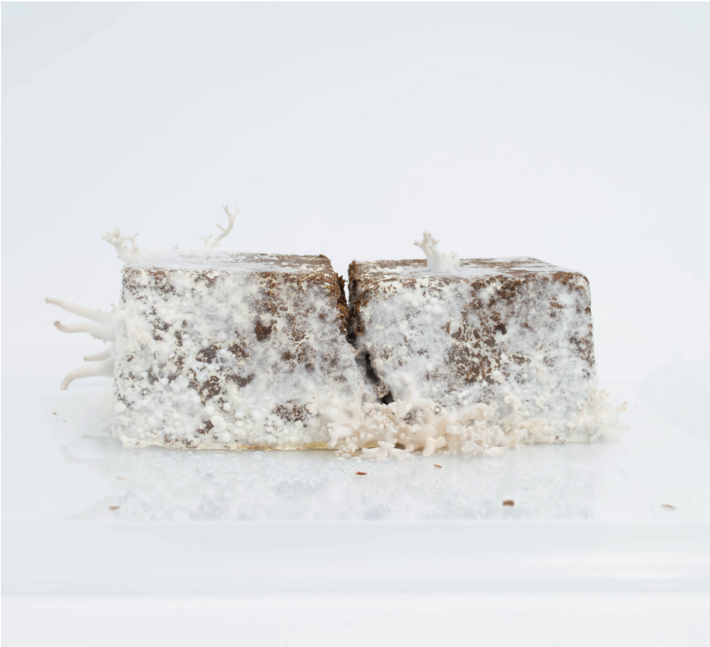
Fig. 15. Fruiting bodies developing on an active mycelium brick (Lab 7.)
