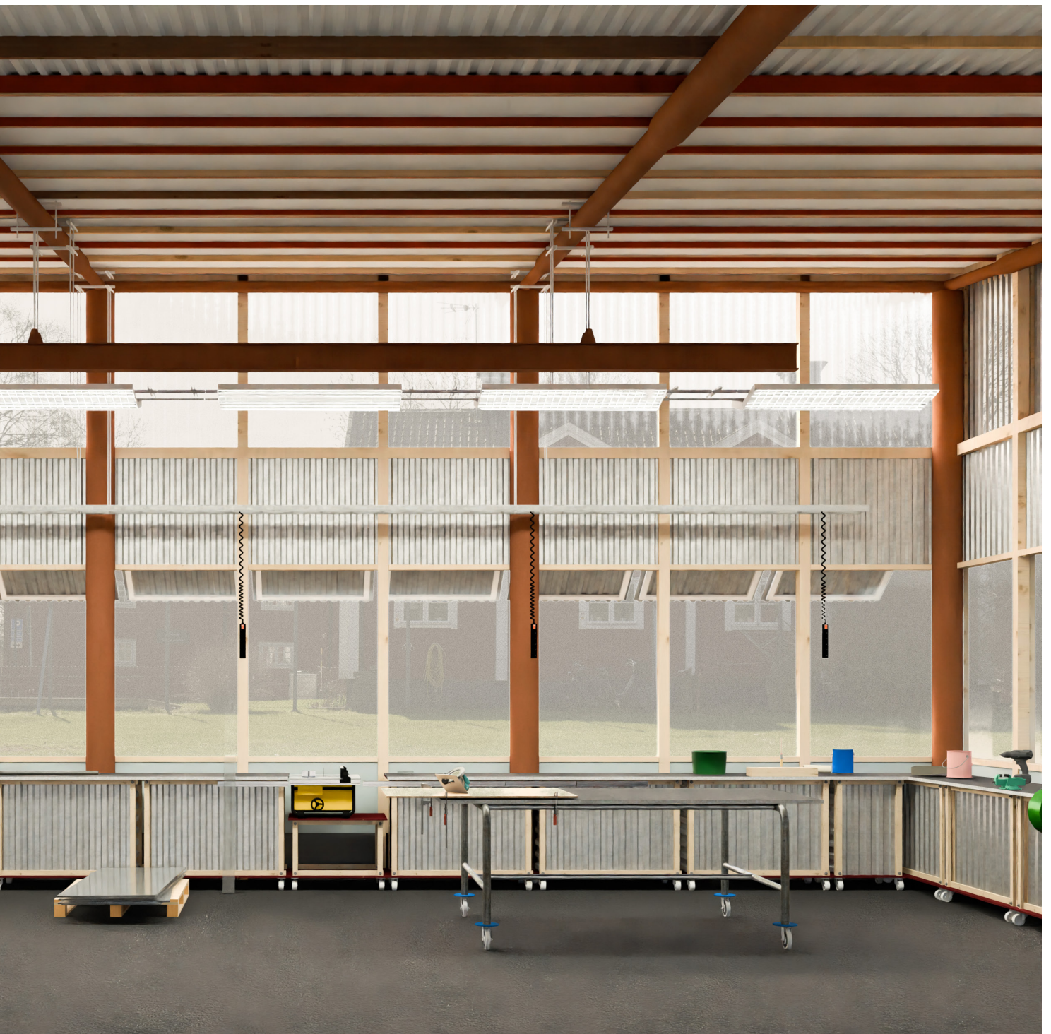
Interior perspective of the workshop. Outside the image is the entrance from the outdoor workshop space and loading zone. To the left of the work bench line is the sink. Then comes the equipment for metal work, then wood and last grinding machine. Above is cable duct with hanging junctions boxes to get a clean workbench from cables.
