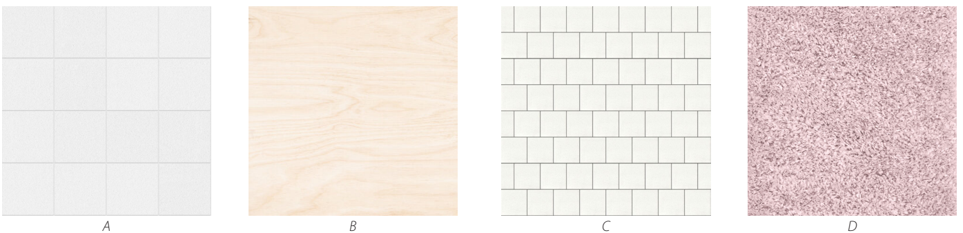
Figure 46. Other materials, standard acoustic square ceiling tiles (A) in every room, with the ability to fasten hooks and hang things from the ceiling in between the squares. A lot of the furniture is made from birch laminate (B), making it a common material the children meet. Tiles (C) are used as a backsplash in the student kitchen and department ateliers with mini kitchens. Textiles, such as carpets (D) are not installed as a permanent architectural component. This is to facilitate cleaning ( when - not if - a child throws up on the carpet it is good to be able to move it immediately, rather than to try to dry it up while making sure no one walks around in it ) and to allow the inhabitants of the space to construct their own rooms, to decide for themselves where a soft carpet should be placed. Textiles are an important sensory experience and can add softness and colour to a room without dominating it.
