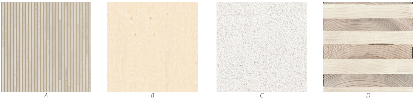
Figure 45. Material for internal walls, a pine acoustic wall (A) covers one wall in the piazza, otherwise plywood sheets (B) and plaster (C) cover most walls. Walls made by CLT (D) have their outer lamellae visible, which looks more like the other plywood walls (B), but can remind and awaken curiosity of the material structure (D). The colours are limited, leaving space for displays of current projects and the children's own art.
