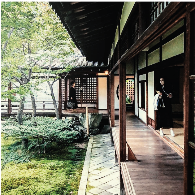
Engawa along the facades of a courtyard. This outer layer of structure and space diffuses the borders between interior space and the nature.
