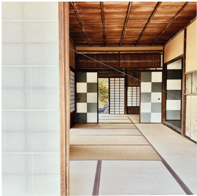
First Tea House, with a clear axis from facade to facade, divisible by sliding shoji- and fusuma screens. It may be open to nature, or closed off in sections.
