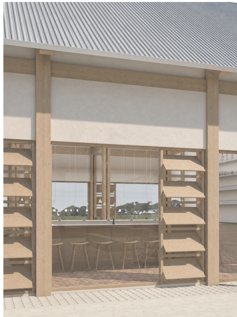
Windows with adjustable wooden slabs for ventilation.
