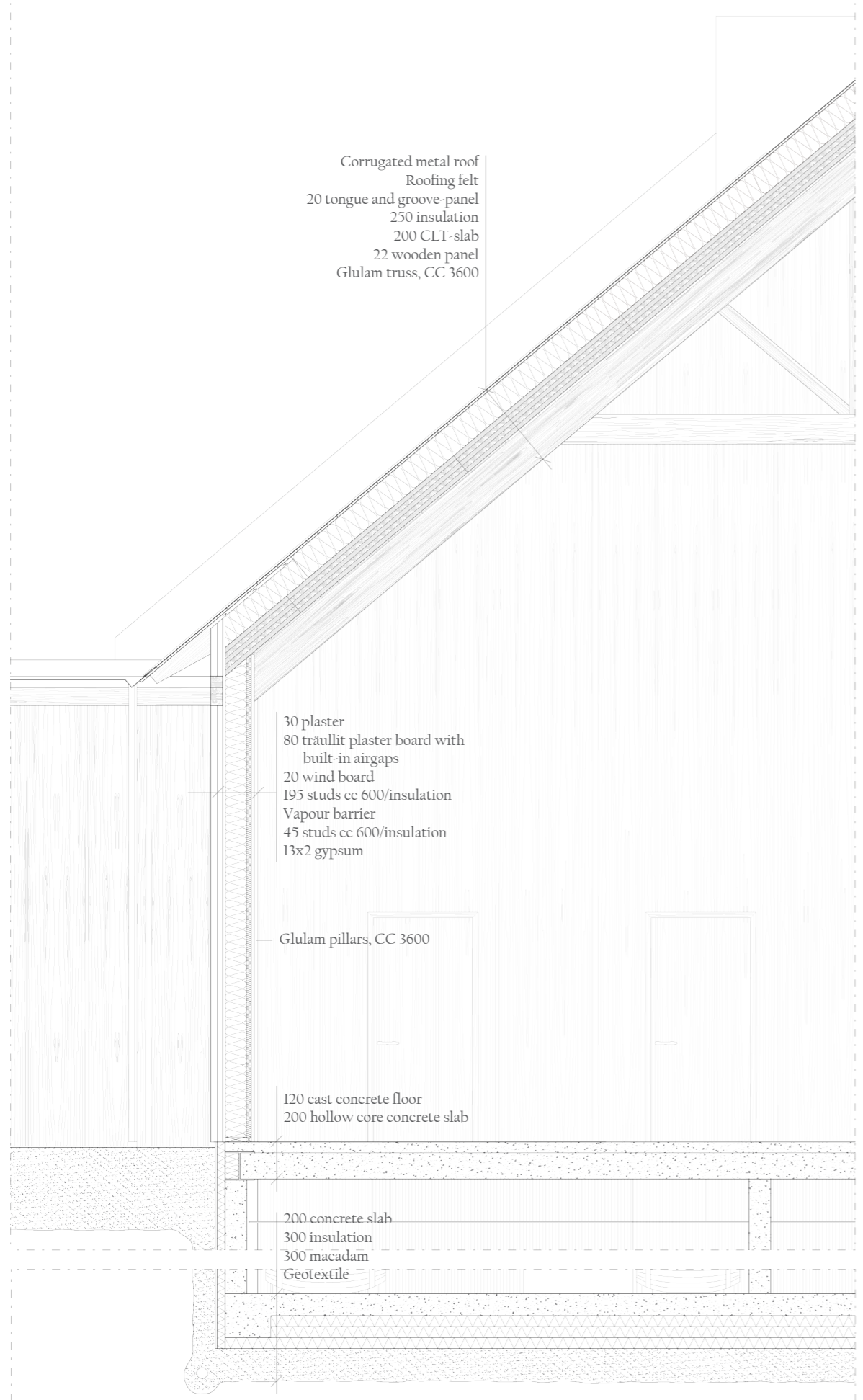
Detail section, production building 1:50 (A4)
