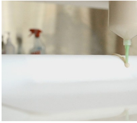
[Fig. 27]→ Syringe (and nozzle) running perpendicular to the XY plane
