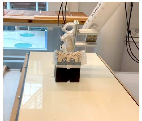
[Fig. 29] → Robot head movements when syringe (and nozzle) runs perpendicular to the mold
