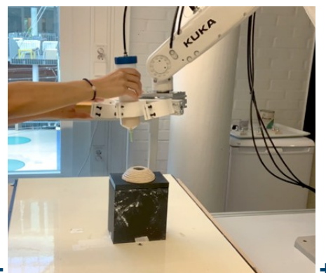
[Fig. 28]← Robot head movements when the syringe (and nozzle) runs perpendicular to the mold, with a controlled angle to avoid robot head collisions.
