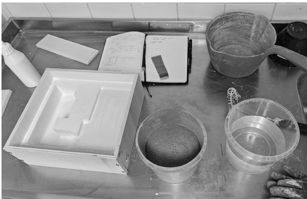
Fig. 29 Model process: assembly of the foam and wooden molds, preparation of the pre-mixed concrete. © Inès Romy
