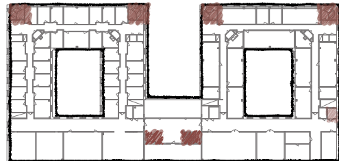
Figure 22: Floor plan showing vertical communication. Akademiska hus. Modified by the author, published with permission.
