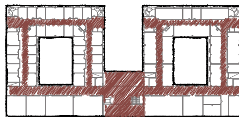
Figure 23: Floor plan showing horizontal communication. Akademiska hus. Modified by the author, published with permission.
