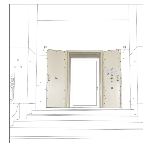
Vault door 2: positioned at the entrance to the small cashier hall. Also communicates trust by visibly suggesting that money is kept safe.
