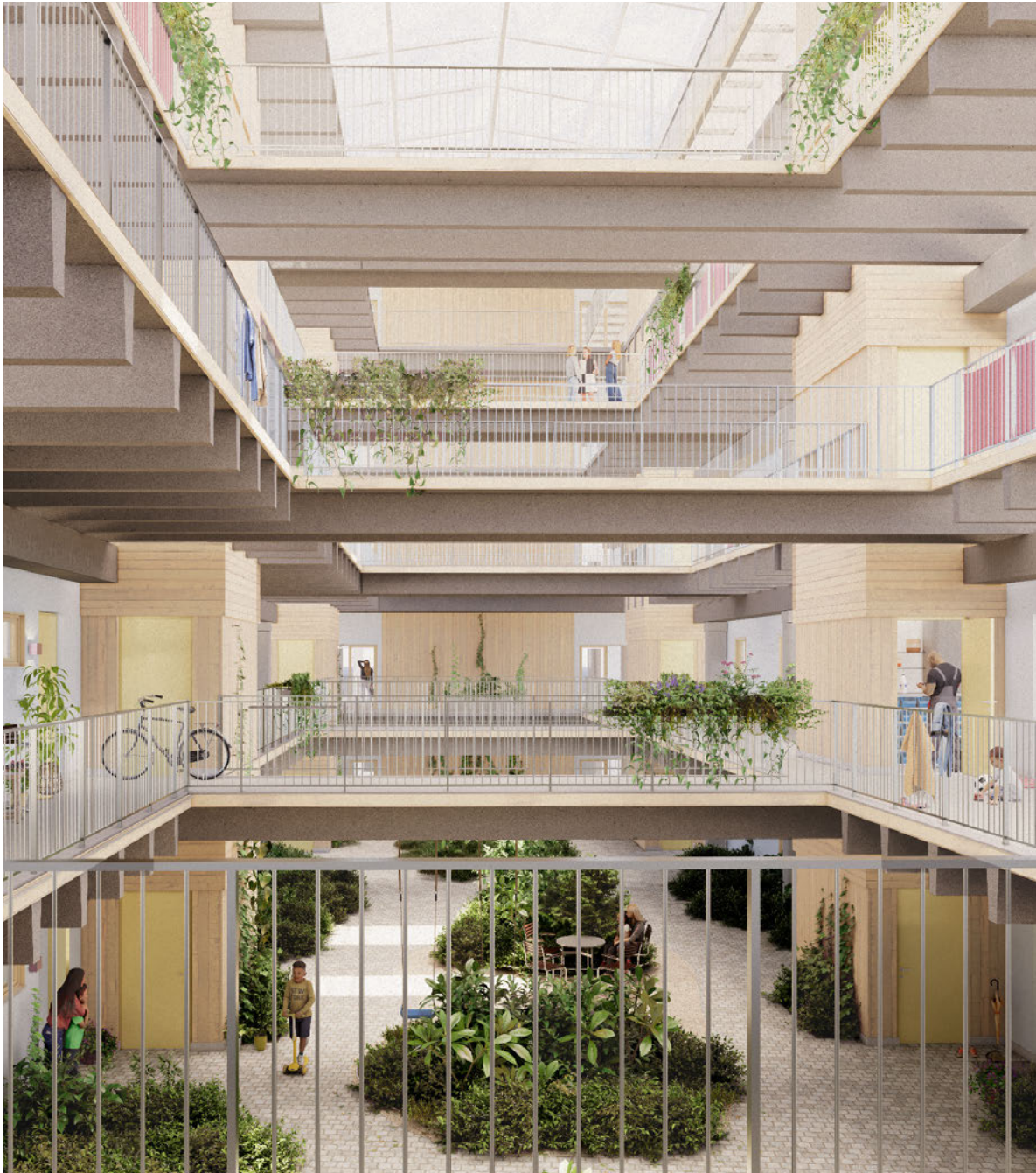
Visualization of atrium. The atriums bring daylight to the dark core and contribute to residential quality and make for an atmospheric sequence when moving through the building. Storage units clad in wood divide the communication zone into sequences and provide a more private zone for the dwellers.
