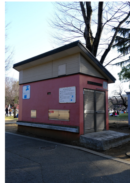
Figure A.5. Emergency water station, connected to a water tank underground, Ueno park.
