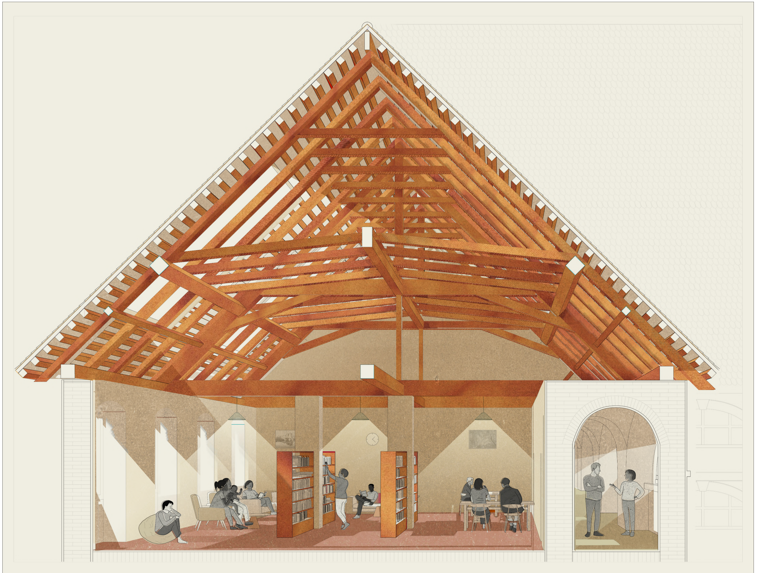
Figure 49: Second floor communal reading space, perspective section
